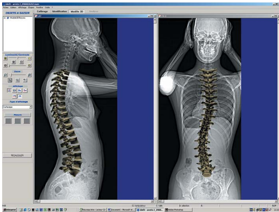
Fig. 7. 2-D radiographs acquired with EOS, a 2D–3D low irradiation dose scanner (3D reconstructions are superimposed)
